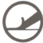
Concrete floors - extend blade with bevel facing up
