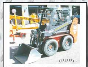
(#34353) 36-inch skid loader, Thomas mdl. 85, 19hp, compact-fits thru gates
